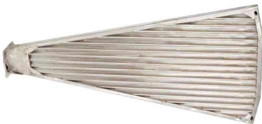
Rebuilt Sector prior to poly media installation
